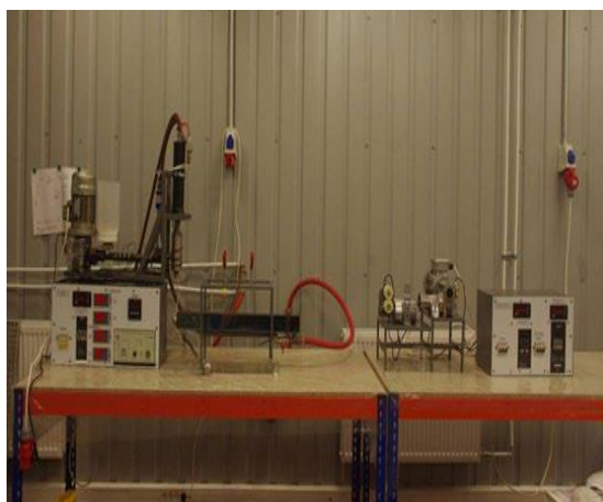
FIGURE 1 Laboratory extruder with the ultrasonic treatment of the melt (know-how of the technology is registered in the FSBEI VO "MGUPP")
