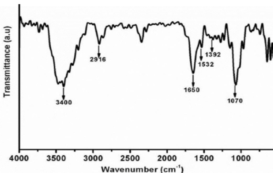
**FIGURE 7** IR spectrum of (AuNps)
