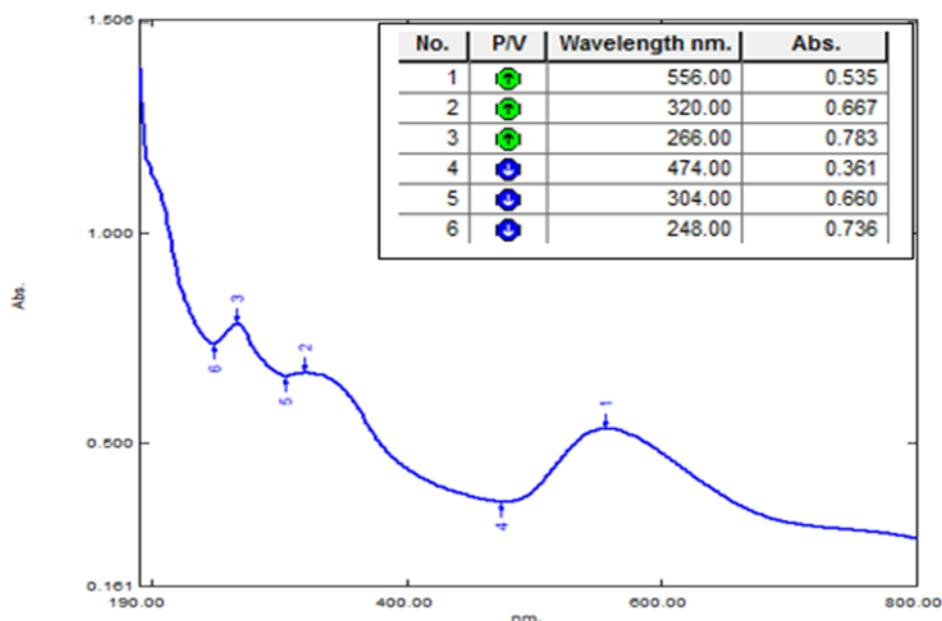
**FIGURE 3** The maximum wavelength of gold nanoparticles
