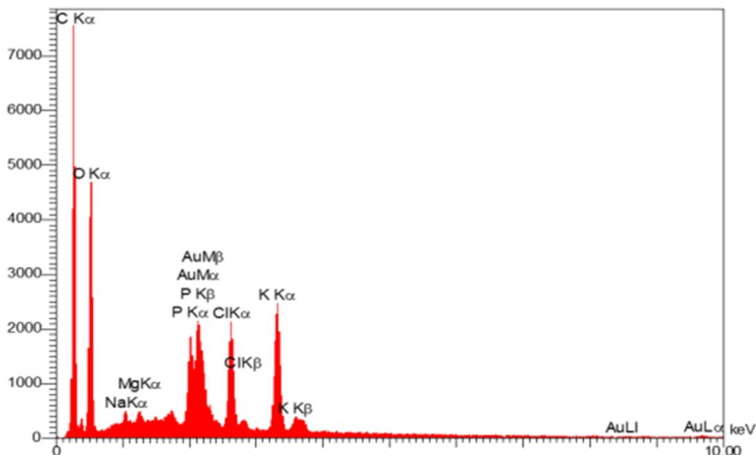
**FIGURE 5** shows the results of the examination of gold nanoparticles using X-ray energy scattering
