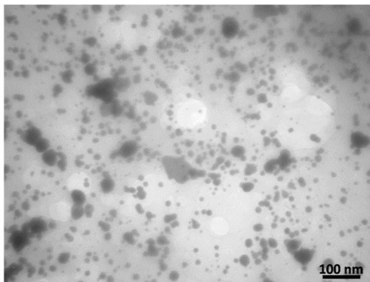
**FIGURE 4** Examination of gold nanoparticles under a transmission electron microscope
