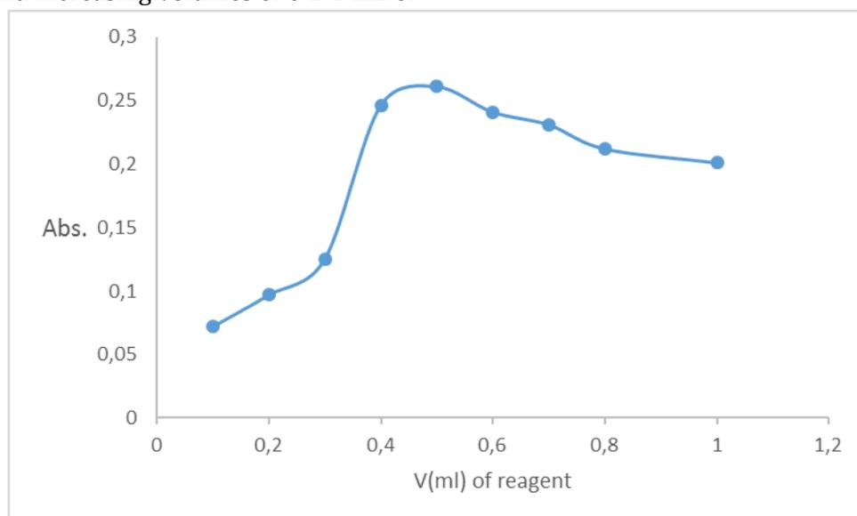
**FIGURE 9** Effect of reagent volume (100 $\mu\text{g}/\text{mL}$ ) DSH on the absorption of the colored complex
