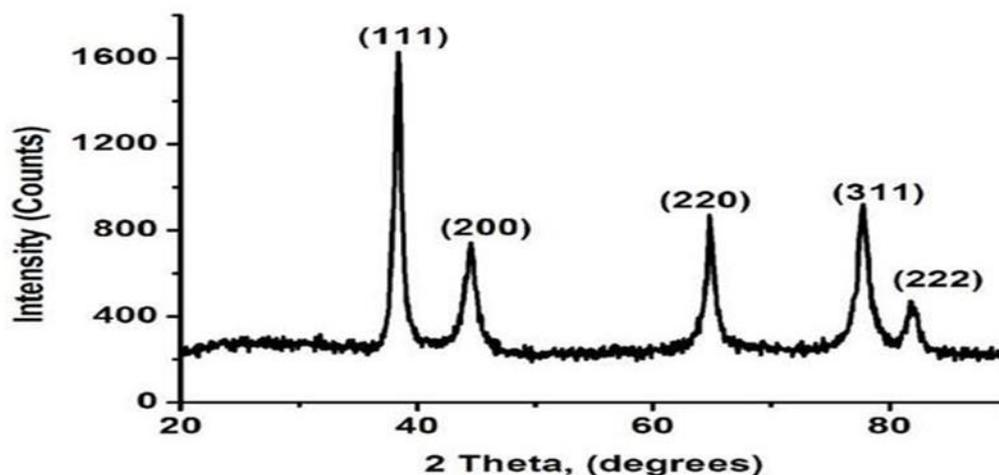
**FIGURE 6** XRD analysis of (AuNps) Crystalline nanoparticles
