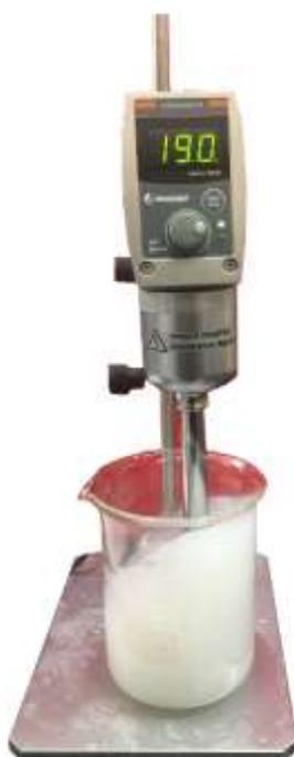
**Figure 1.** Mechanically homogenization with 26000 RPM
