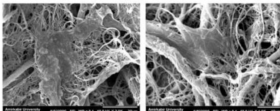
**Figure 5.** SEM images of cell adhesion on the silk nano-fibres
