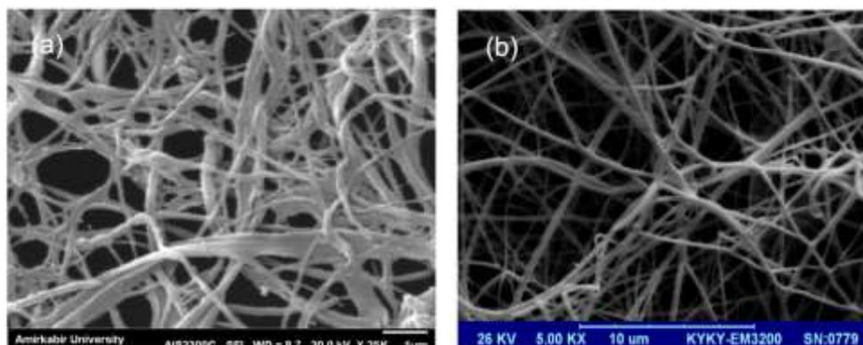
**Figure 4.** SEM images of silk nano-fibers prepared by (a) old chemical method (b) novel physical method
