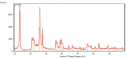
**FIGURE 3** XRD spectrum of kao/Al surface
